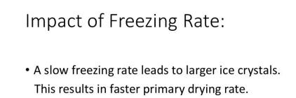
• A fast freezing rate leads to smaller ice crystals. This results in a slower primary drying rate
